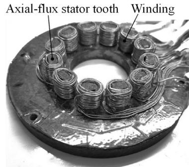
Fig. 8 Fabricated axial-flux stator.
