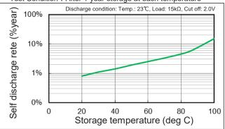
Note: The self-discharge rate of less than 20°C shows the same self-discharge rate as 20°C.
