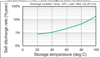
Note: The self-discharge rate of less than 20  $^{\circ}\!\! C$  shows the same self-discharge rate as 20  $^{\circ}\!\! C$  .
