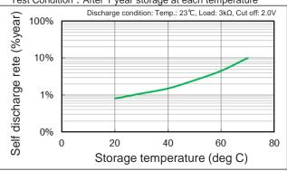
Note: The self-discharge rate of less than 20℃ shows the same self-discharge rate as 20℃.
