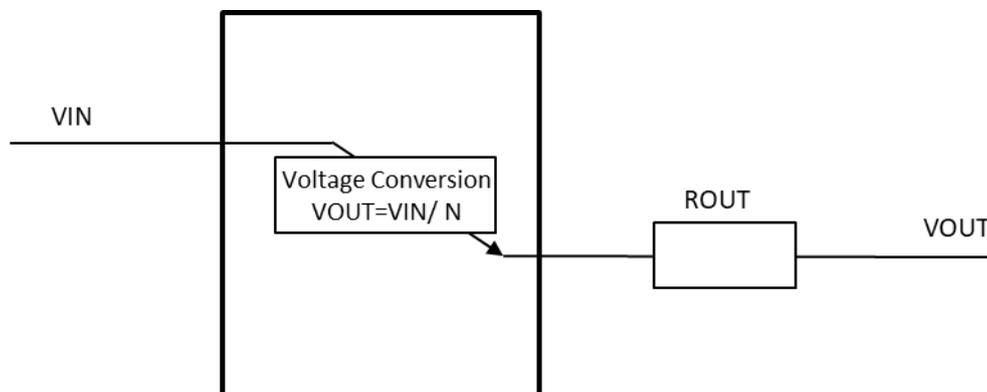
Figure 3. Idealized diagram for charge pump
