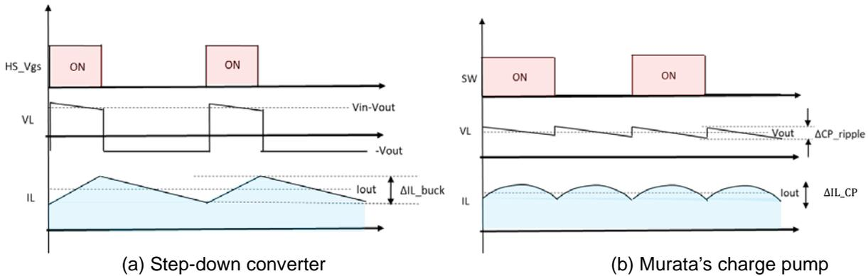
Figure 5. Inductor voltage and ripple current
