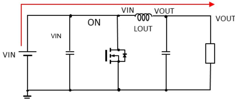
Figure 4. Step-down converter (State 1: High side FET ON)
