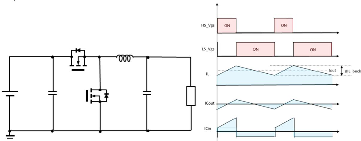
Figure 2. Step-down converter
