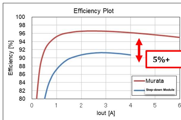
Figure 7. Efficiency characteristics (VIN=48V, VOUT=12V)
