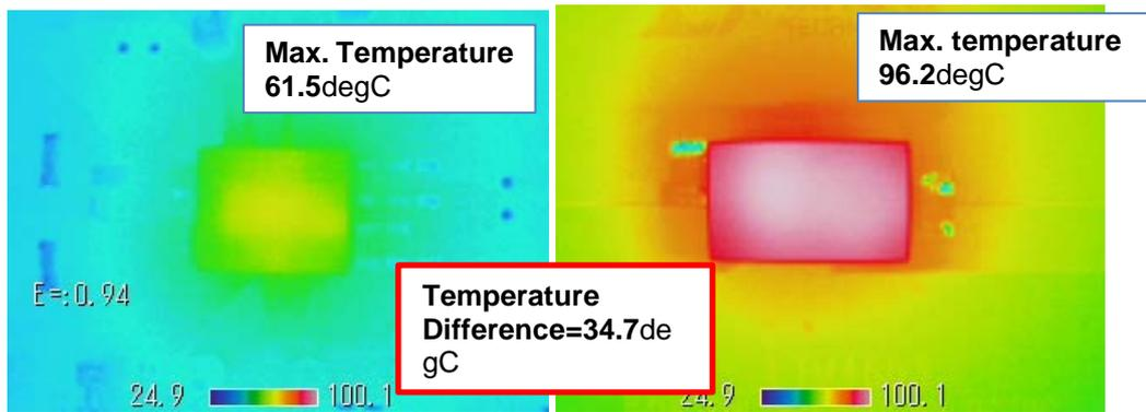
Figure 9. Temperature characteristics (VIN=48V, VOUT=12V, IOUT=4A)
