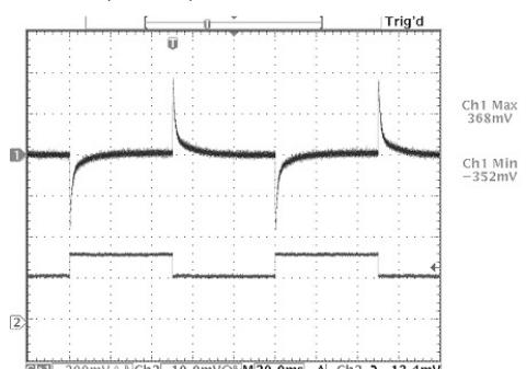
$V_{IN}=48V$   $I_{OUT}=3A-4A$   $C_{OUT}=240\mu F$
