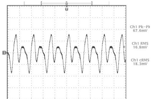
$V_{IN}=48V$   $I_{OUT}=0.81A$   $C_{OUT}=240\mu F$
