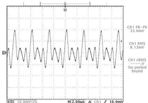
$V_{IN}=48V$   $I_{OUT}=3.81A$   $C_{OUT}=240\mu F$
