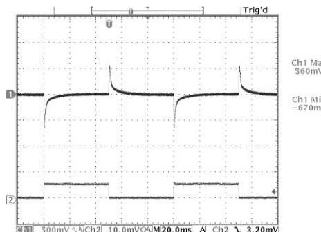
$V_{IN}=48V$   $I_{OUT}=1A-2A$   $C_{OUT}=240\mu F$
