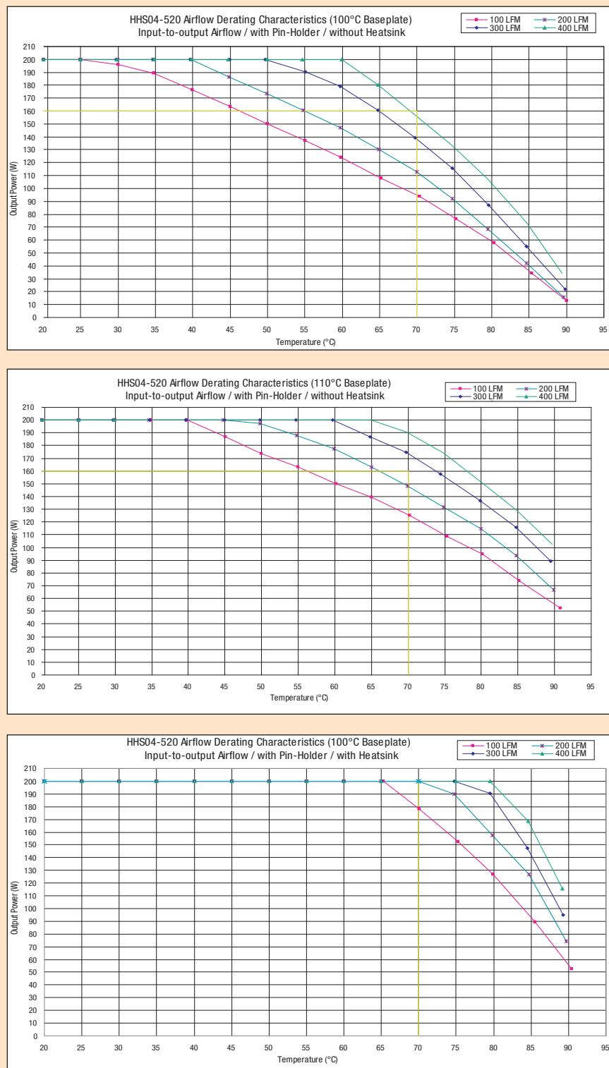
Heatsink used is 2.28" L x 2.4" W x 0.7" H, non-anodized, mounted to baseplate, where noted above.
