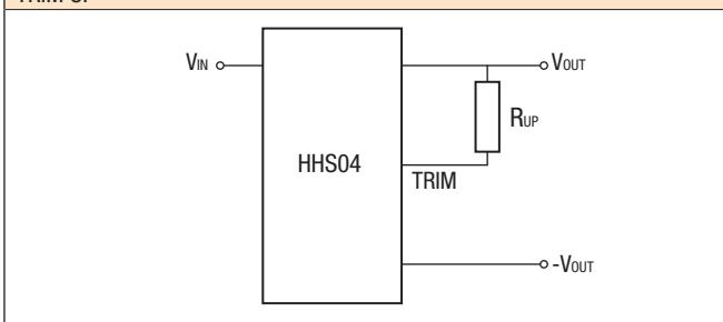
When the output voltage is trimmed up, output current must be derated so that the maximum output power (shown in the selection table) is not exceeded.
