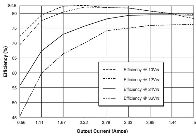
Figure 2c. Efficiency vs. Output Current and Input Voltage
