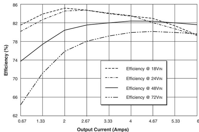
Figure 3c. Efficiency vs. Output Current and Input Voltage
