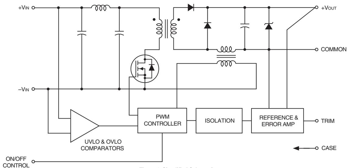
Figure 1. Simplified Schematic
