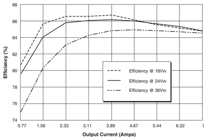
Figure 4c. Efficiency vs. Output Current and Input Voltage
