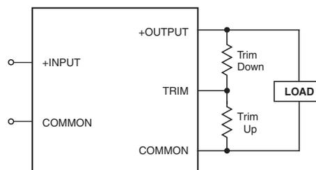
**Figure 8. Trim Connections Using Fixed Resistors**
