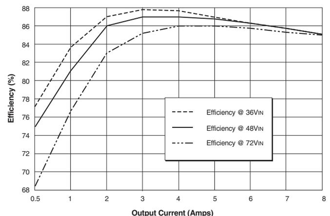
Figure 5c. Efficiency vs. Output Current and Input Voltage
