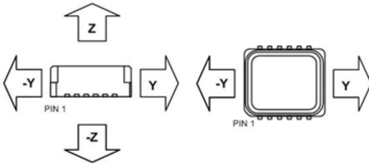
Figure 3. Accelerometer measuring directions
