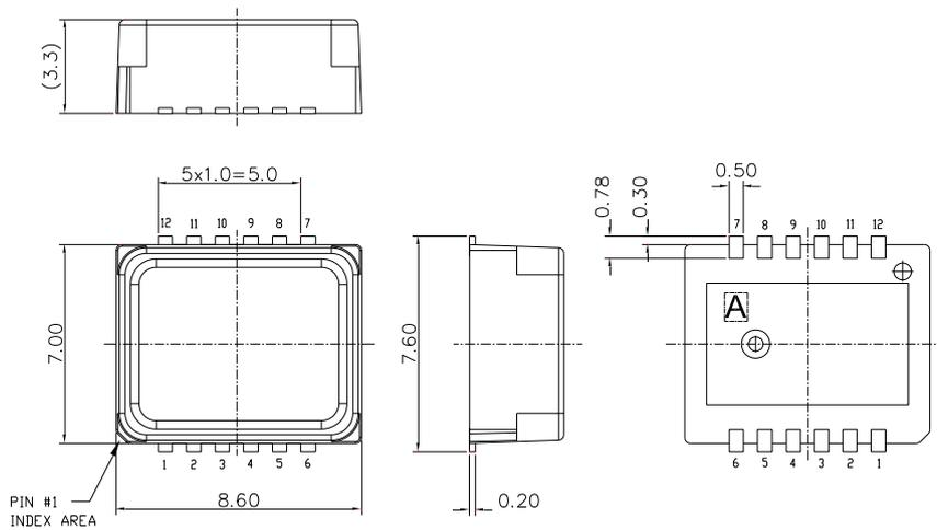
Figure 4. Housing dimensions
