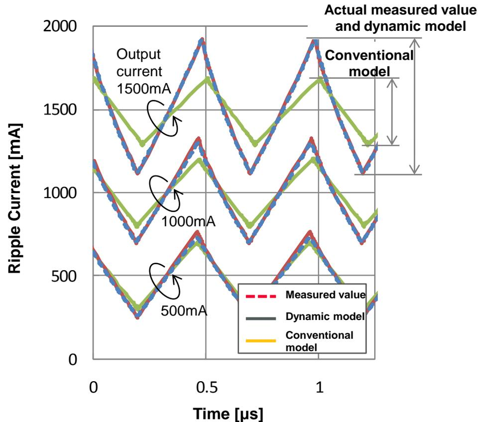
=> In a conventional model, since the current dependent characteristics of an inductor are not reflected, the simulation results deviate from the measured value. On the other hand, in a dynamic model, results close to the actual measured value could be acquired.
