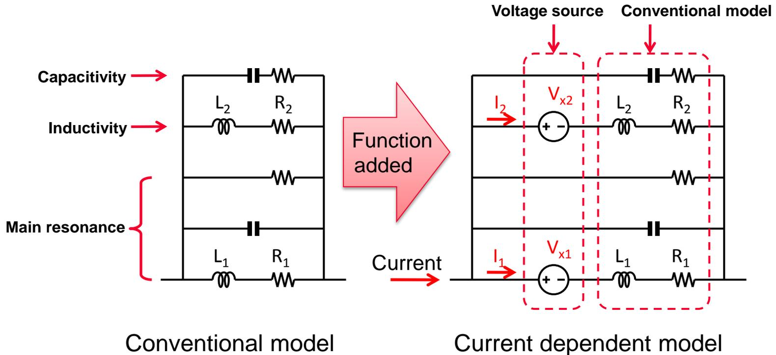
=> Adding current dependency to several components of a conventional model, realized a dynamic model which responds to the change of inductance along with the change of the real time current.
