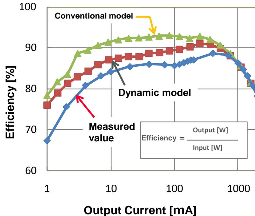
=> In the simulation by a dynamic model, results closer to the actual measured value could be acquired.
