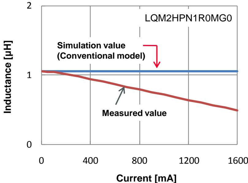
=> The DC superposition characteristics are not reflected in the (1) conventional model.
