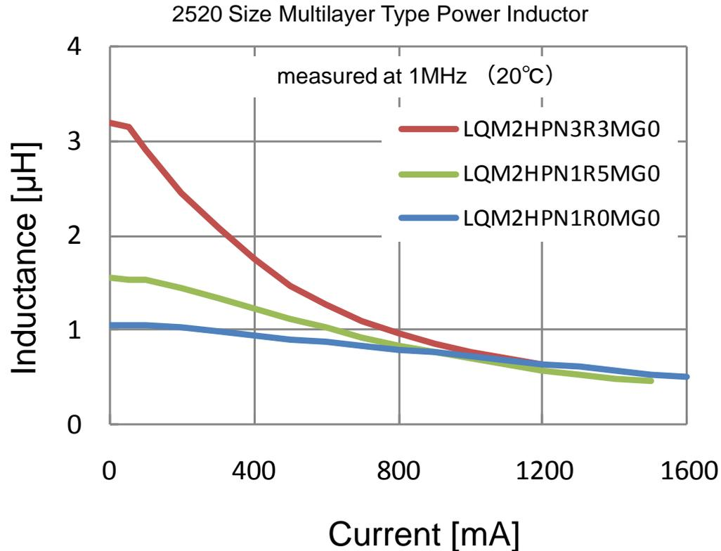
=> In ferrite based power inductors, when a large current flows through, since the ferrite approaches magnetic saturation, the permeability decreases during the process. The inductance also decreases because the inductance is proportional to the permeability. The above figure shows the characteristics (**DC superposition characteristics**) when a direct current flows through a power inductor.
