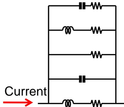
=> Even when the current changes, the constant of each component does not change (DC superposition characteristics are not reflected)
