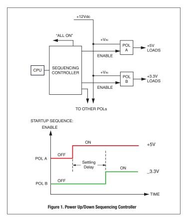
fast-rising, all-or-nothing step which may be unacceptable to certain circuits, especially large output bypass capacitors. These could force POL's into over-current shutdown. And some circuits (such as many linear regulators and some POL's) may not have convenient start-up controls. This requires designing and fabricating external power controls such as high-current MOSFET's.
