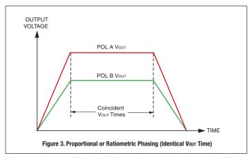
Figure 3 shows two POL's with different slew rates in order to reach differing final voltages at about the same time.
