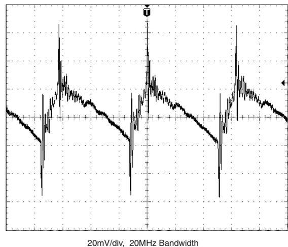
**Output Ripple and Noise of BWR-5/700-D48A**
