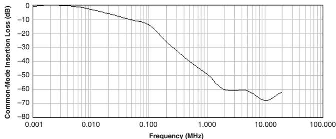
**FLT-100V20 Common-Mode Insertion Loss**
