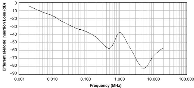
**FLT-100V20 Differential-Mode Insertion Loss**
