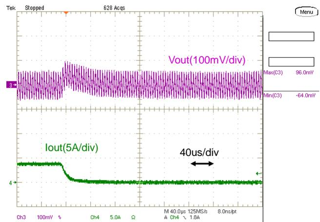
Fig.12-2-36. Load Transient Response (Io= 3.5A → 0)
