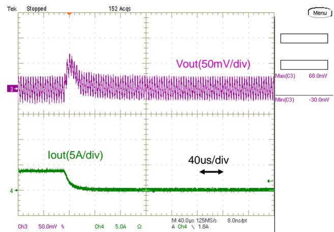
Fig.12-2-12. Load Transient Response (Io= 3.5A → 0)
