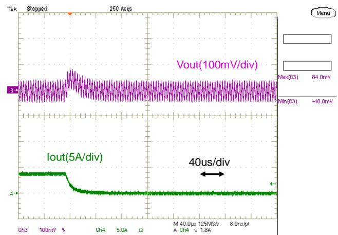
Fig.12-2-30. Load Transient Response ( $I_o = 3.5A \rightarrow 0$ )
