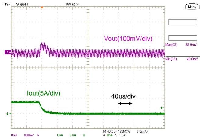
Fig.12-2-24. Load Transient Response (Io= 3.5A → 0)
