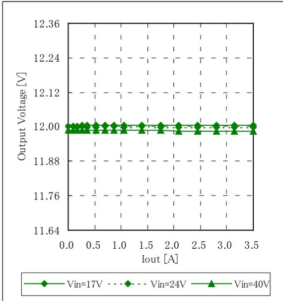
Fig.12-1-4. Output Voltage vs. Output Current
