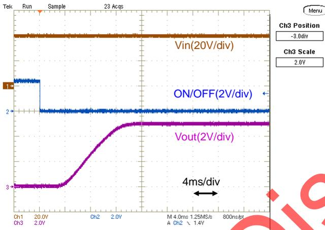
Fig.12-2-15. Start-up Waveform (Io=0A)
