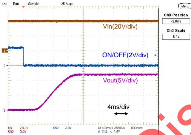
Fig.12-2-33. Start-up Waveform (Io=0A)
