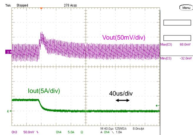
Fig.12-2-18. Load Transient Response (Io= 3.5A → 0)
