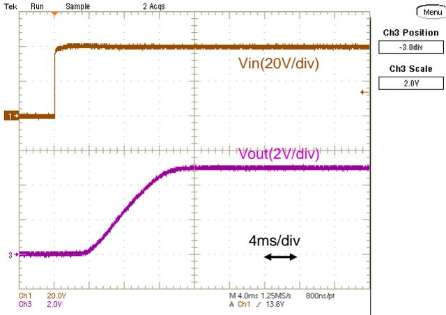
Fig.12-2-13. Start-up Waveform (Io=0A)
