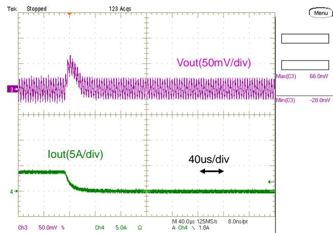
Fig.12-2-6. Load Transient Response (Io= 3.5A → 0)
