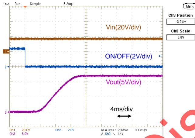
Fig.12-2-21. Start-up Waveform (Io=0A)
