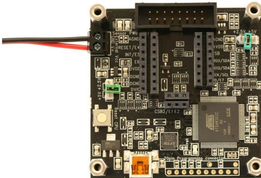
Figure 46. Evaluation board with external power cable inserted
