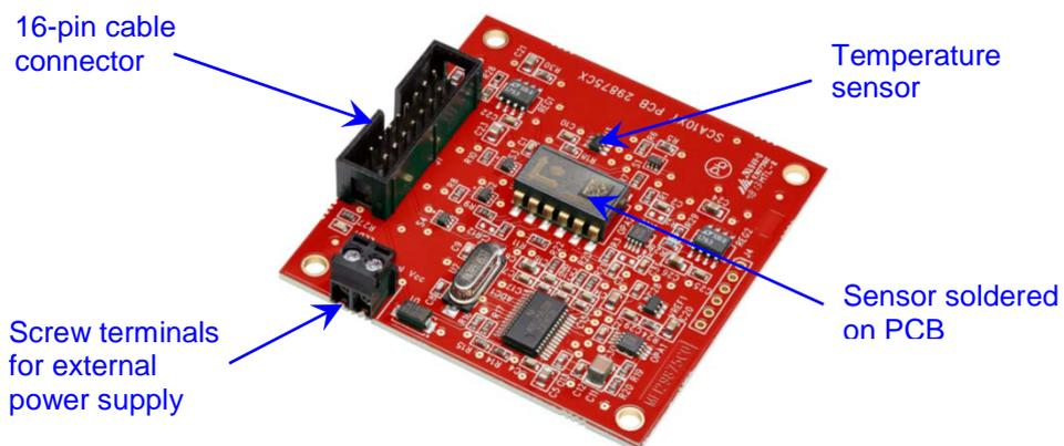
Figure 2. Extension board (SCA10xT PCB)
