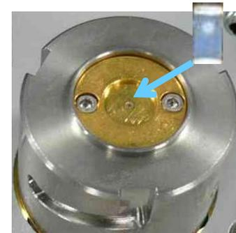
Insert into the measurement opening with the direction identification mark facing up.
