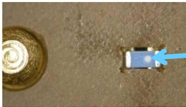
Insert with the direction identification mark facing to the right.
